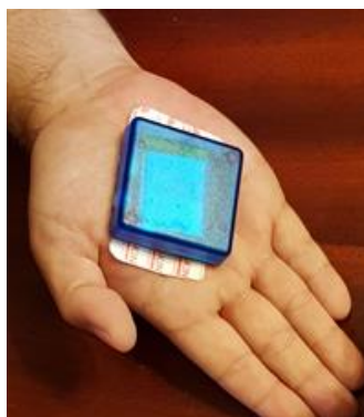
Open-source Bio-Monitor (OBIMON) for electrodermal measurement (K. Kasos et al., 2019) used in Study 3.
